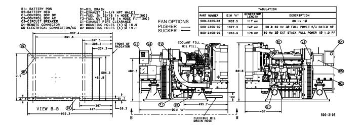
Note: This outline drawing is provided for general reference only and is not intended for design or installation. For more information see Operation and Installation manuals or obtain drawing 500-3105 and wiring diagram from your distributor/dealer.
